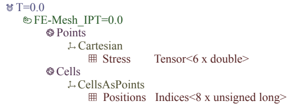
Figure 4: F5 layout of a C3D8 element's integration point data. One exemplary stress data field is stored in the 'Points' skeleton. No 'Points' 'Positions' field is required as integration point coordinates can be computed from the nodal grid.
